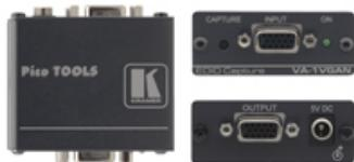
The VA-1VGAN is an EDID emulator for computer graphics video signals. The unit can capture an EDID setting in non-volatile memory from the output allowing convenient and reliable connection to the source
